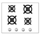
Poor mapping: arbitrary arrangement of stove controls
